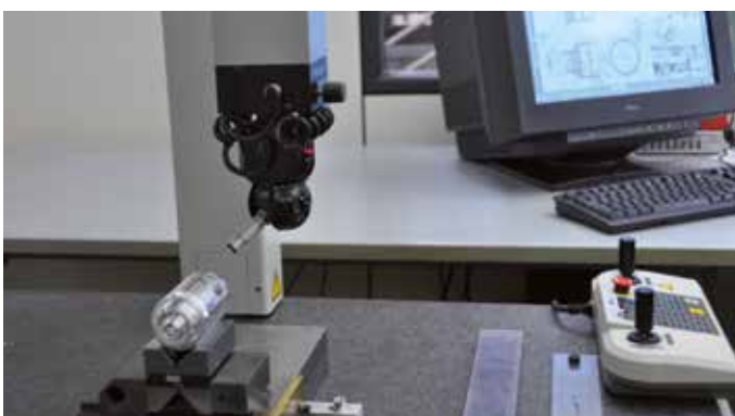
Inspection of a hydraulic pump core by 3D device
